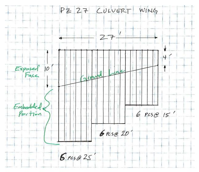
Wing shall be installed as close as possible to existing barrel. Wing shall be removed and disposed of in an approved waste site. Fabric shall be placed on the backside, between the barrel and the wing to provide a seal and then flowable fill shall be poured to fill the void. Fabric is incidental to other items of work as detailed herein. Concrete shall not contact waters of the project. Any spalling shall be patched. Patching is incidental and shall be made using approved materials.
